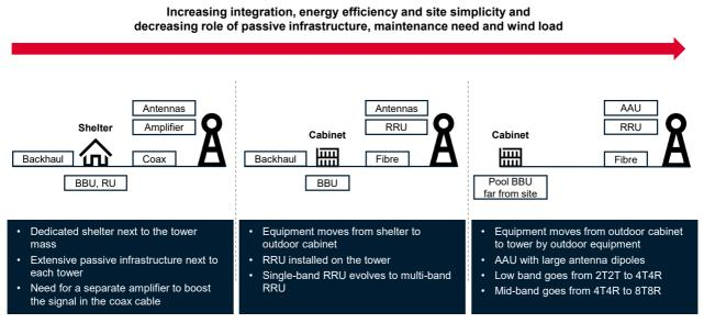
Baseband unit (BBU), radio unit (RU), remote radio unit (RRU), active antenna unit (AAU)
